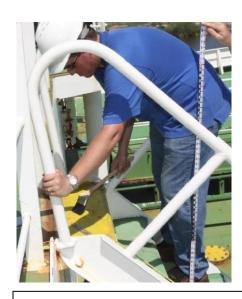
In a case involving a seaman's fall on a merchant vessel, a mechanical engineer used the above images to show the relative size of the seaman (represented by a chief mate who was of similar size and build) to explain that the seaman did not fall from a ship's ladder in the manner he claimed.
